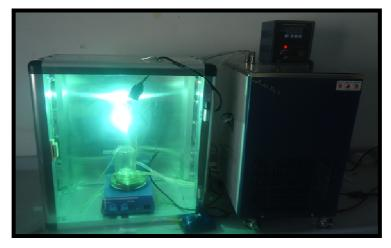
**Plate1**: the unit that used in the photo decolonization of Congo red dye by use the new prepared couple semiconductor.
