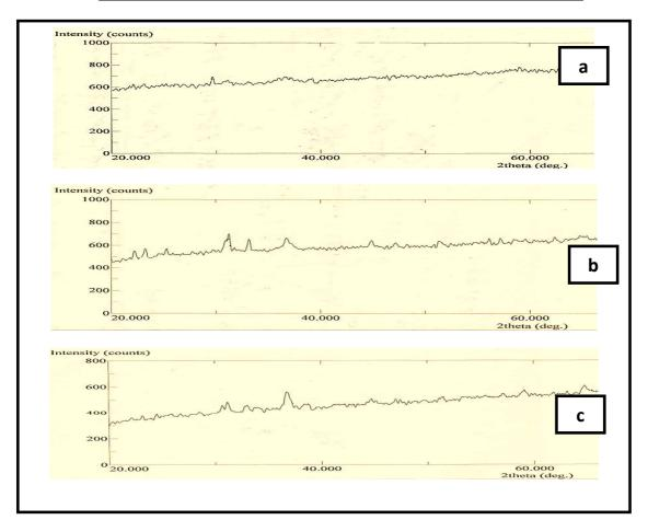
**Fig.1**. XRD patterns of the prepared coupled oxides powders calcinated at different temperatures 300  $^{\circ}$ C Fig.a, 500  $^{\circ}$ C Fig.b, and 700  $^{\circ}$ C Fig.c .
