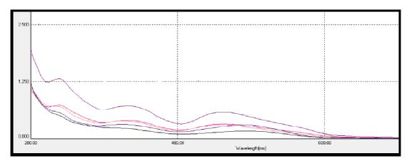
**Fig.2**. Photocatalytic declorization of congo red dye using 0.15g of  $(Cr_2O_3-Co_2O_3)$  calcienated at 700°C.
