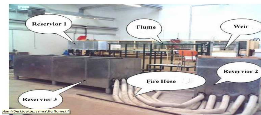
Fig.1:the experimental flume of the 60° bend related to Akhtari (2009) [12]
