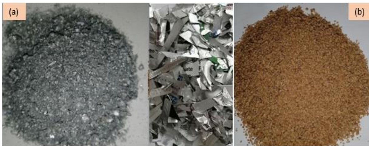
Fig .1: Filter media (a) aluminum foil, (b) husk of walnut
